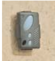
Left: A wall mounted transmitter is provided that may be removed, if required, from its cradle.
