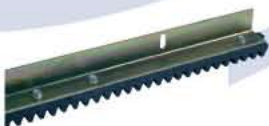
ACS9000 Module 4 RACK (sect. 25x22mm) in Nylon with right-angle (up to 1000 kg) in 1mt bars ACS9001 Set 10 m
